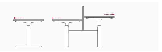
Top displacement (13 cm). Total accessibility to the electrification canal. Allows the displacement of double table tops and single tables towards the user, allowing easy access to the electrification channel. Optional on double tables: A larger lower channel with sheet metal covers is incorporated for housing and continuity of electrical systems.
