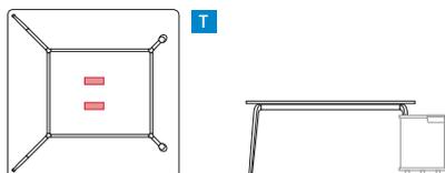
TWIST Desk **TWS4441000T** finished in white melamine surface and desk edge, white structure and levelers, with 2 "T" access to wiring centred on the desk.
