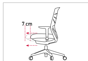
7 different positions. Depth adjustment with self-return mechanism
